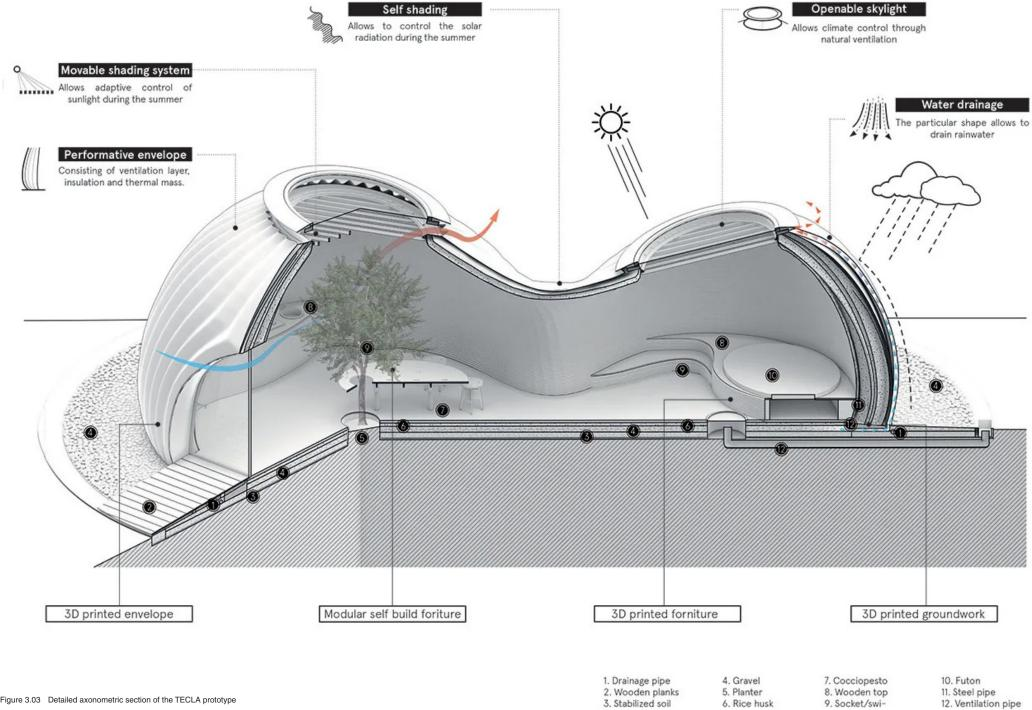
Figure 3.03 Detailed axonometric section of the TECLA prototype
