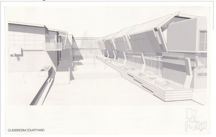
The classroom courtyard is flanked by classroom wings on two sides and the corridor on the north side. The wing to the right side holds the garden and the sidewalk along the edge of the building. The left holds the benches and the ramp to get to the level below. The courtyard is on two different levels so that a space is delineated if the teachers only want the students to play in a specific area. On the far left is a detail of how the basketball court and hoop would connect to the school.
