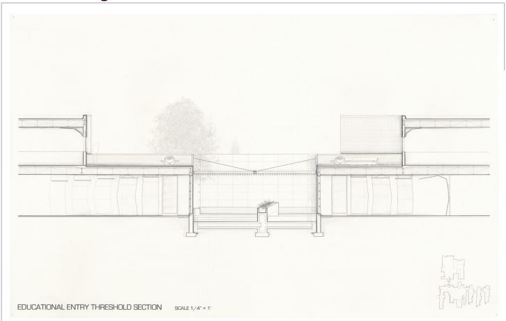
This section is cut through the threshold to the education courtyard. On the right is a computer lab and on the left is an art room. On the second floor are classrooms that have a connection to an outdoor terrace. The terrace like the other outdoor areas holds places for seating and for planting. In the middle of the section is the awning used to demarcate the parking from the educational courtyard.
