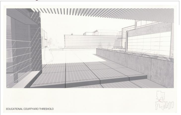
The threshold into the courtyard is put in place to separate the courtyard from the parking lot without the use of a wall. This space is meant to feel like it is encapsulated and secure from the town outside of the school. The awning above wood be created from the same wood that is used on the wraps. On the left in the distance of this rendering is the entrance for the middle school. The right side is the glass that walls in the art room.
