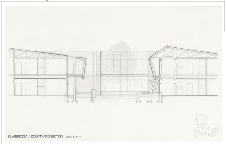
This section shows the connection between the indoor and outdoor of the classrooms and courtyards. The halls are single loaded with classrooms on each level. The left side shows the balcony that is used for plantings.
