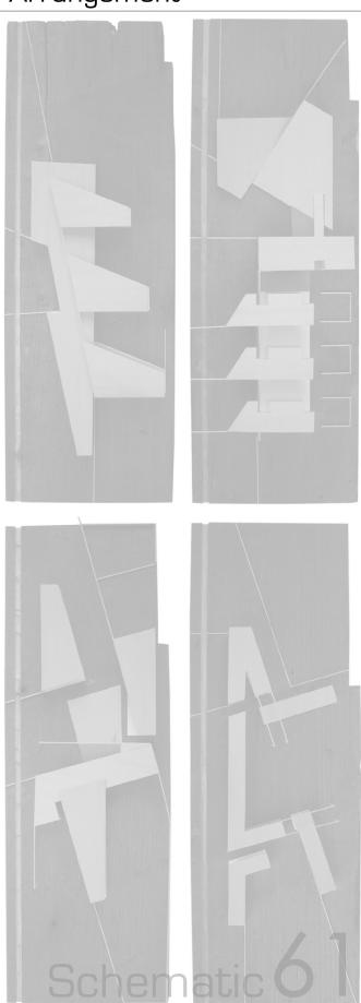
The first model is set up as a house plan. All three schools are located on the back of the campus for security reasons. The core building is on the front so that it can be located closer to the city. This will keep access to the school separate from the students. The saw tooth pattern allows the schools to have openings to the outside with allows for the protection and the indoor/outdoor connection that where experimented with in the previous models.
