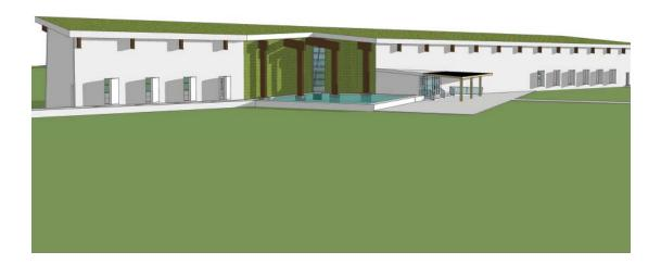
Where the reservoir cuts into the North face of the building the glu-lam structure remains to be exposed and the two angled walls that form the cut are to be build as vegetated living walls to contrast with the pieces of the building that are unaffected.
