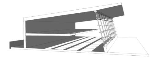
This is a study of a more ecological section for future attempts at the project's form. It is designed specifically so that the section protects the glass from the summer sun while allowing the winter sun to penetrate deep into the building providing for passive solar heating.
