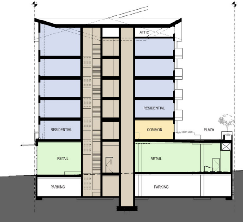
North-South Building Section
