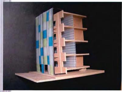
During hours of operation the curtain wall would have the ability to open at the bottom and allow pedestrians to flow into the space directly from the sidewalk, encouraging interaction with the building and the school.
