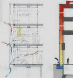
Movement of natural ventilation thru the cavity.
