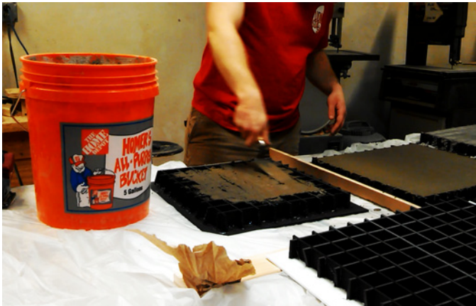
▲ Top: Video still of preparing strips to assemble the grid form from. Bottom: Video still pouring concrete into molds. ▼
