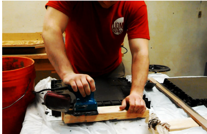
▲ Top: Video still of vibrating the mold to get the concrete into every tight corner.
