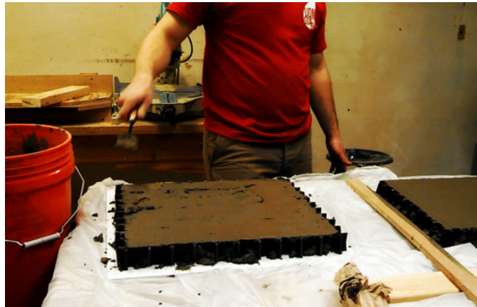
▲ Top: Video still of vibrating the mold to get the concrete into every tight corner.
